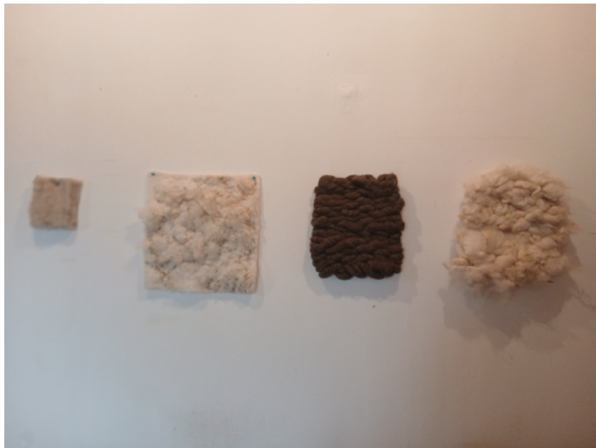
Four samples of wool insulation, 2024–2026, showing (from left to right) commercially produced wool insulation, felted wool, commercially woven wool, and locally woven wool.
